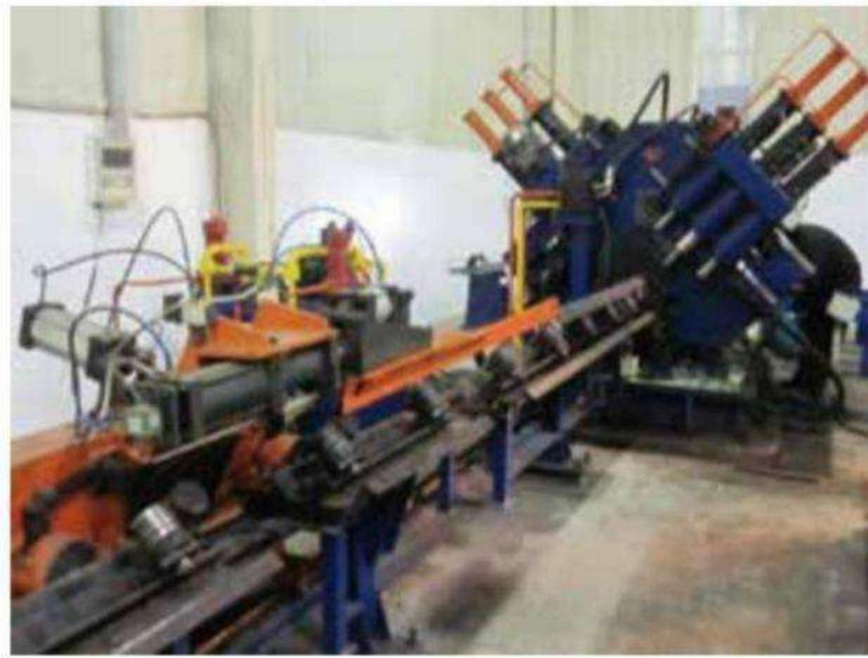
▼ 角钢钻数控生产线 CNC angle steel drilling production line
